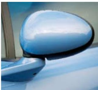
**Above:** Mirrors were lifted from Rover 75, but with different bases.
